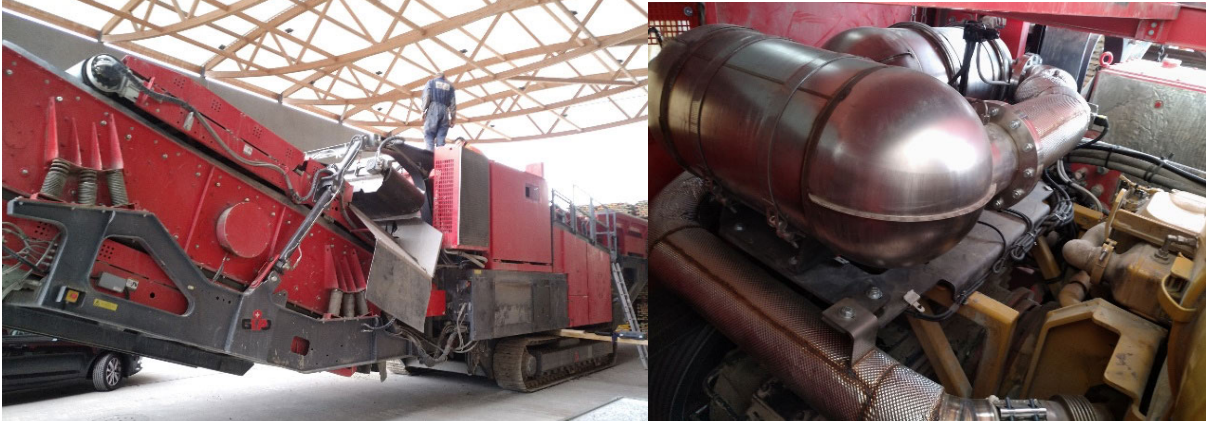
Figure 15: Gipo Stone Crusher - CH Caterpillar C-13; 354kW @ 2200rpm Stage IIIa, Stage V Target, Airless-Dosing System
